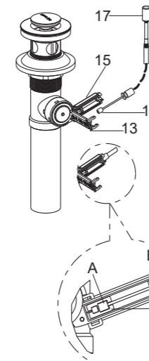
Open the coverplate(13) on the drain body, and insert cable end(14) into the square hole(16) of the cable box(15). Make sure the cable is properly buckled at both ends(A, B) of the cable box as the figure shown.
